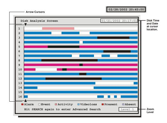
Rotating the **Jog** moves the two arrow cursors across the representation of the recorded video. As the cursors move across the screen the corresponding disk time is indicated in the upper right of the screen. The video representations are color-coded by category. Rotating the **Shuttle** expands (Zooms) the display. The Lowest level (most detail) is indicated on screen with an **(L)**. Pressing the **Enter** button will start Playback from the cursor location.
